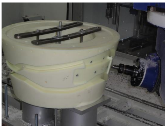
Figure 7 – Example Products – Poultry Farming Machinery - Machining 5-axis
