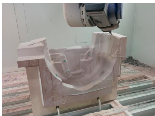
Figure 8 – Example Automotive Products – Machining 5-axis
