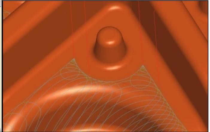
**Above – Adaptive Area Clearance** - All the machining moves have lead in/out arcs to maintain a smooth machine motion. The cutting moves are also smooth, flowing profiles without sudden changes of direction.
